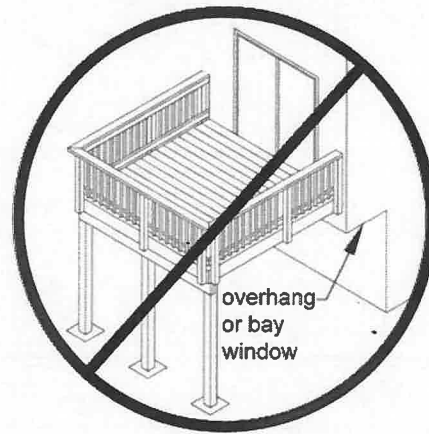
Figure 18. No Attachment to House Overhang with Ledger.
